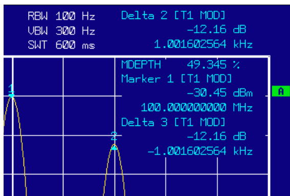
Fig. 5-10 Measurement of the AM modulation depth. The modulation depth shown is MDEPTH = 49.345%. The frequency of the AF signal can be obtained from the frequency display of the delta marker.
